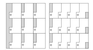
Using design to reduce scrap: designing parts so that they nest closer to one another is a way to maximize sheet utilization.
