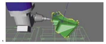
**Production simulations** | Many types of design and programming software enable users to simulate production. This allows design engineers to test sheet metal parts as often as necessary to identify problems. Today, computer simulation has become an indispensable pre-production tool, particularly for the manufacture of complex parts.
