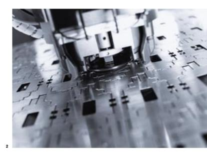
**Everything on the punch press** | When solid parts are substituted by sheet metal parts, these parts often still require machining of some kind. Holes still have to be drilled, and threads have to be cut. The most cost-effective solutions, however, do not require any cutting at all. This can be done, for example, by using the punch press to form threads instead of cutting them.
