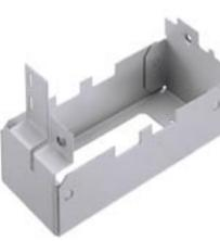
2 Microjoints: thin support pieces keep punched parts from falling out of the sheet skeleton.
